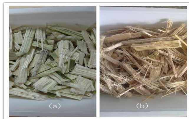
Figure 5. Quality comparison of oil palm frond using (a) Spouted bed (b) direct sunlight.
