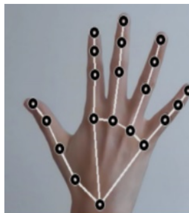
Figure 2. The black dots correspond to the joints detected in a hand using Google's Mediapipe library.
