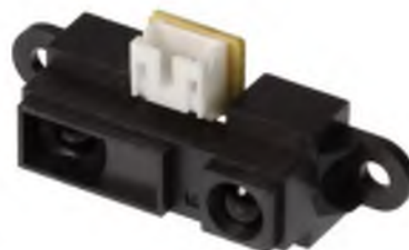
Figura 4.5: Sensor Infrarrojo GP2Y0A21YK0F.
